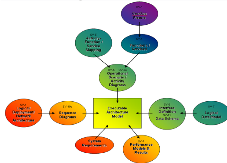
Figure 3 shows required elements of integrated architectures to provide a concept of operations picture, activity-functions service mapping, functions/services, and operational activity diagrams.
